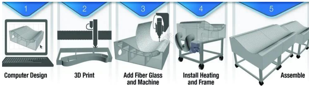
Figure 4. Process for 3D printing wind turbine blade molds
