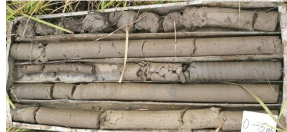
ZK80 (1.2–0.5 m) pulverized clay layer (3-2 layers, plastic)
