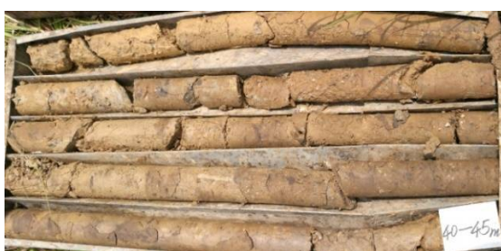
ZK176 (40-45m) pulverized clay layer (4-2 layers, hard plastic)
