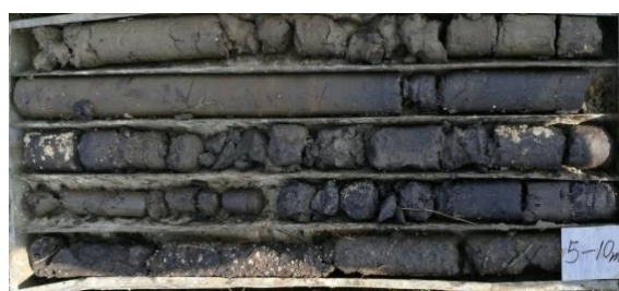
ZK70 (5–10 m) Silt-bearing clay layer (3-4 layers, plastic)
