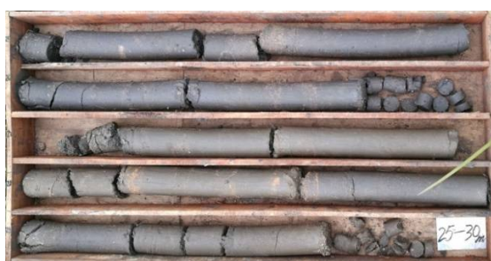
ZK110 (25–30 m) pulverized clay layer (3-5 layers, hard plastic)
