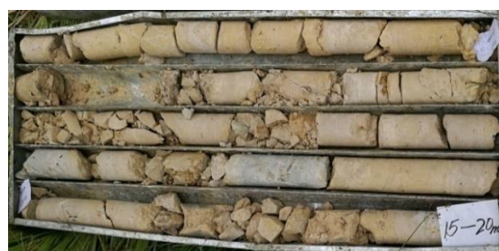
ZK26 Moderately weathered limestone (layer 5-3)
