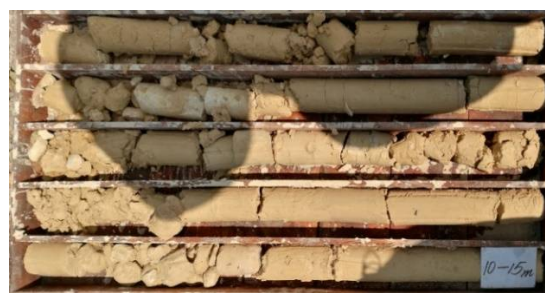
ZK1 fully weathered limestone layer (5-1 layers)
