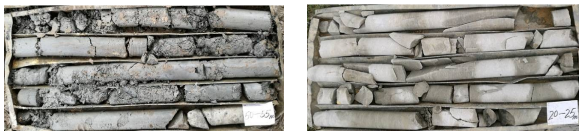
ZK75 Strongly weathered marl layer (layer 6-1)
