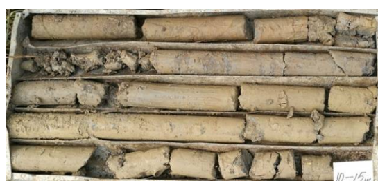
ZK97 (10–15 m) pulverized clay layer (layer 4-1, plastic)
