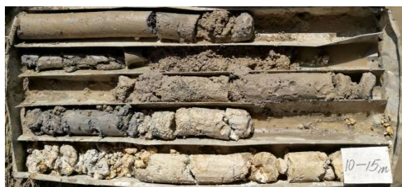
ZK95 (11.6–13.4 m) medium-coarse sand layer (3-3 layers)
