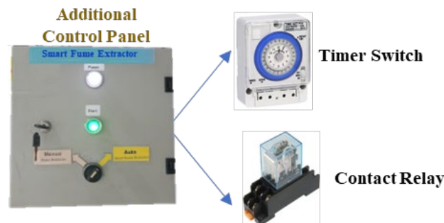
Fig. 6. Components on additional panel.
